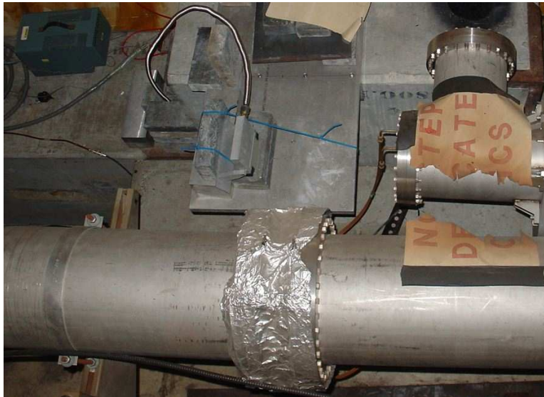
Figure 3: The prototype Quartz fiber detector installed at SLAC. Synchrotron radiation from the ESA bend magnets exits from the port shown at the right. The PMT box is installed below the beam line in a shielded cave.
